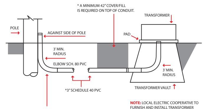
ALL PRIMARY TO BE CONSTRUCTED WITH ONLY ELECTRICAL 90° ELBOWS and 45° ANGLE FITTINGS, SHALL BE NO MORE THAN 3-90° ELBOWS OR COMBINATION THEREOF. FOR EXAMPLE, 1-90 AT THE HOUSE, 1-90 AT THE POLE OR TRANSFORMER, 1-90 or 2-45'S CAN BE INSTALLED IN THE REMAINING CONDUIT. ALL RISER ELBOWS TO BE SCH. 80 PVC.
